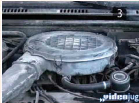
Fig : Cleaning of air filter housing
